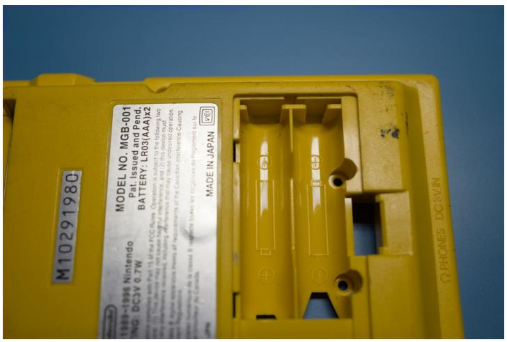
Now with the battery terminal removed, we can cut the shell.
