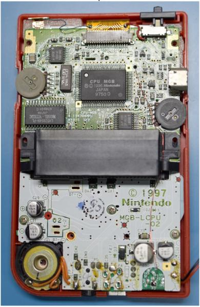
Route the wire against the board, around the cart slot, and into the hole that's above and left of the CPU
