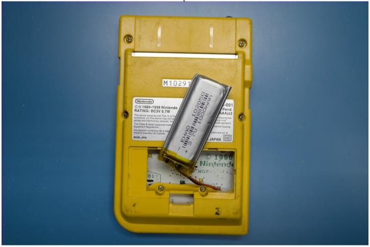
place the rear of the shell on the front of the shell while routing the battery through as shown. Install the 6 triwing screws.
