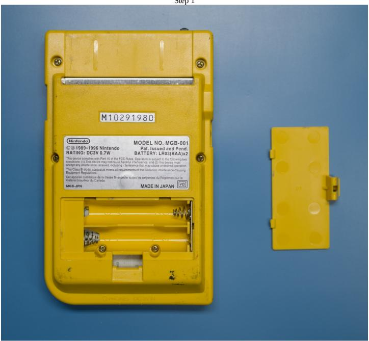
Remove battery cover to expose two screws underneath. Remove all 6 screws using triwing screwdriver.
