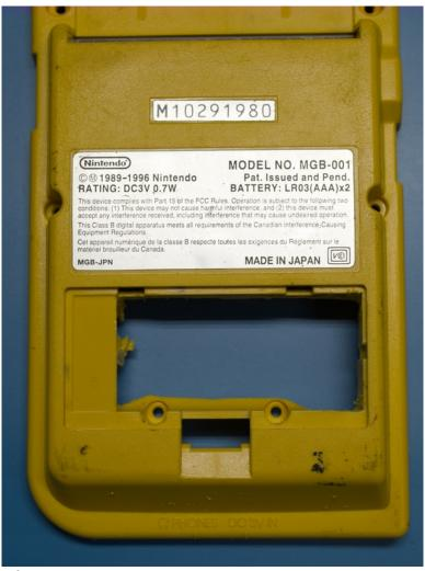
Using the cutting tools of your choice, cut the area shown out. Be sure to leave the two screw holes intact.
